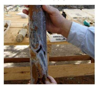
Left: Drill core from Cerro di Oro showing quartz stockwork. Gold-silver mineralization at La Gitana is associated with multistage quartz stockworks, breccia-veins, and locally as disseminations.
