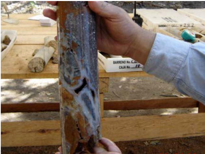
DRILL CORE FROM LA GITANA DRILLING SHOWING QUARTZ STOCKWORK.
